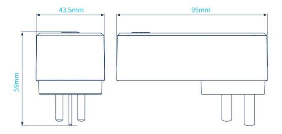
Dimensions (Length x Width x Height): 95mm x 43.5mm x 59mm
